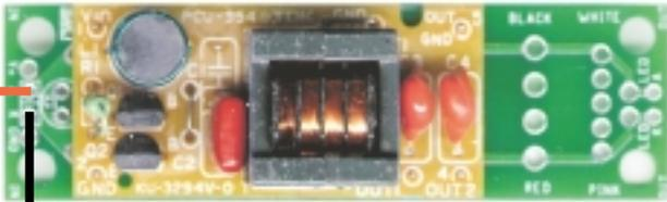
These Lines Power the Inverter Used to Drive the Backlight on CCFL Displays Under Software Control. Match K and A Directly to Display on LED Backlit Displays.
