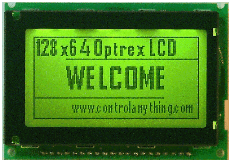
The Optrex DMF50427 LCD Display with LED Backlight controlled by the GDCO-DMF50427 RS-232 LCD Display Controller Chip.
