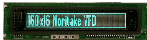
Noritake GU160x16-800 controlled by our GDCN-GU160x16-800 controller chip.
