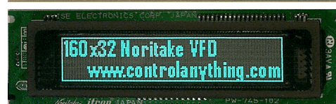
Noritake GU160x32-800 controlled by our GDCN-GU160x32-800 controller chip.
