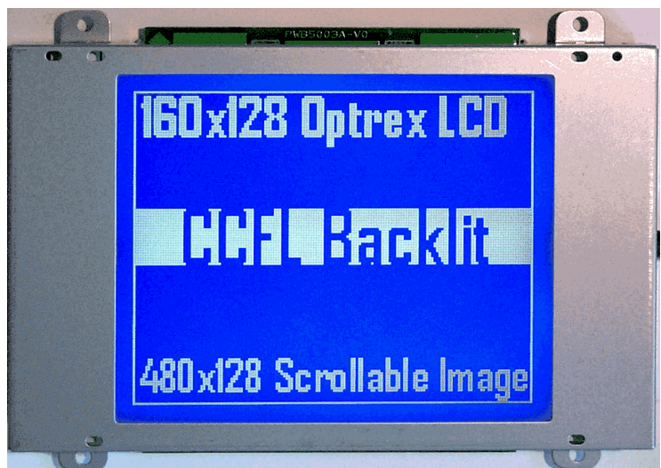
The Optrex DMF5003 LCD Display with CCFL Backlight controlled by the GDCO-DMF5003 RS-232 LCD Display Controller Chip.
