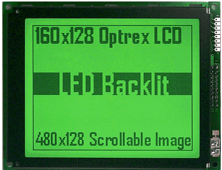
The Optrex DMF5001 LCD Display with LED Backlight controlled by the GDCO-DMF5001 RS-232 LCD Display Controller Chip.
