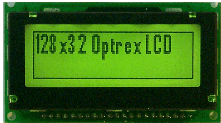
The Optrex DMF50426 LCD Display with LED Backlight controlled by the GDCO-DMF50426 RS-232 LCD Display Controller Chip.
