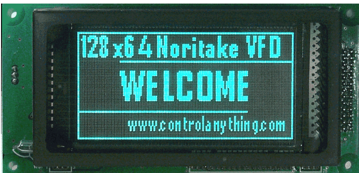
Noritake GU128x64-800 Vacuum Fluorescent Display controlled with our GDCN-GU128x64-800 controller chip.
