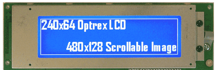
The Optrex DMF5010 LCD Display with CCFL Backlight controlled by the GDCO-DMF5010 RS-232 LCD Display Controller Chip. This display is very similar to the DMF5005, with the exception that it uses a 20x1 single in-line header rather than a 2x10 dual-row header. Detailed information on the backlight inverter is available from Optrex USA.
