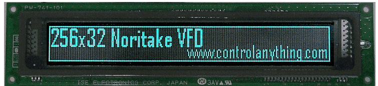
Noritake GU256x32-800 Vacuum Fluorescent Display controlled with our GDCN-GU256x32-800 controller chip.
