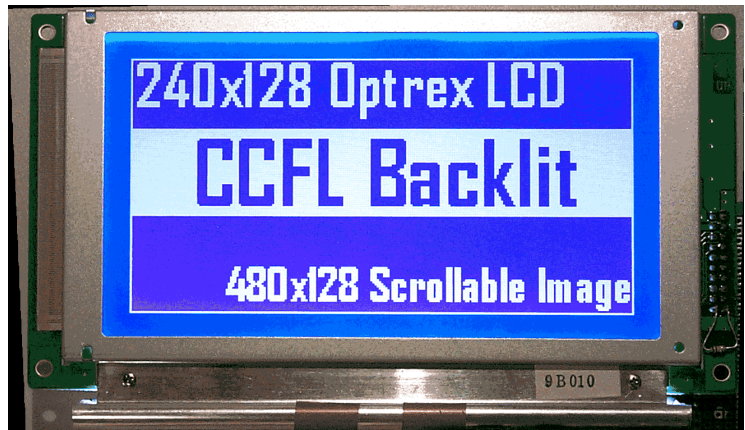
The Optrex DMF50773 LCD Display with CCFL Backlight controlled by the GDCO-DMF50773 RS-232 LCD Display Controller Chip.
