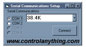
Set the com port and communication rate as shown above. Unavailable COM ports will be ghosted. COM ports 3 and 4 were not available to the ILU when the image above was taken, but may be available on your system. Set the baud rate to match the jumper settings on your display controller. For best results, set to 115.2K baud. Once set, click the "Connect" button. If two-way communications was established with the display controller, a windows similar to the one shown below will appear:
