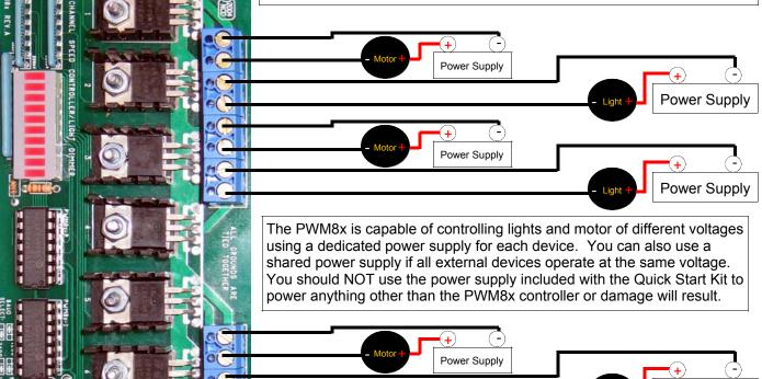
The PWM8x works by controlling the length of time an external load, such as a light or motor, is connected to ground. The more time the device is allowed to be connected to ground, the more power the external load will appear to have. The PWM8x provides 256 levels of speed control for motors and 256 levels of brightness control for light bulbs.
