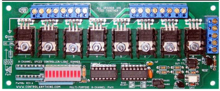
PWM85 Shown Above is an Ideal Solution for many computer controlled motor speed control and light dimming applications.
