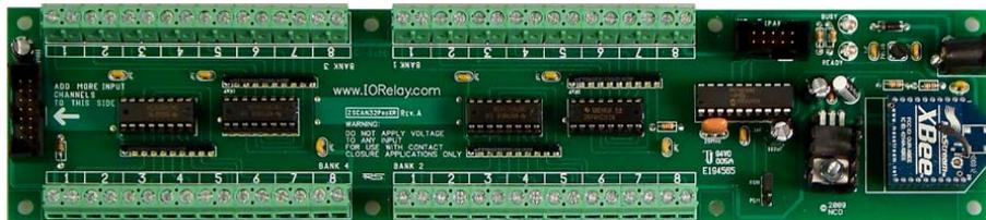
**ZSCAN32 MIRROR** 32-Channel Contact Closure Input ZigBee Mirror Module
