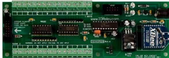
**ZSCAN16 MIRROR** 16-Channel Contact Closure Input ZigBee Mirror Module
