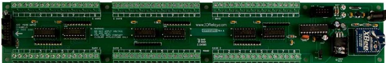
**ZSCAN48 MIRROR** 48-Channel Contact Closure Input ZigBee Mirror Module
