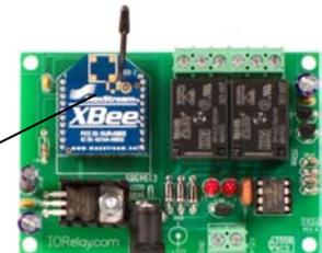
Step 6: Remove the ZigBee Module from each relay controller. The complete serial number is shown at left with a red Box around it. You only need the LAST 8 DIGITS of the serial number. In the case of the module shown, you will need 40018E66. Logging your serial numbers will be critical to proper configuration.
