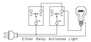
**MirC/MirX Users:** Two contact closure inputs in the sender board and either of the inputs can control one light or device.
