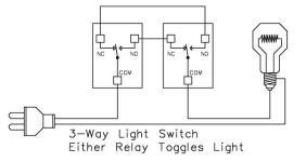
relays at one time is like flipping 2 switches at once....with the same result. This sample is particularly useful since you can replace one relay (as shown in the diagram) with a physical light switch. This will allow a computer to control a light as well as manual operation of a light. Properly used, this can be one of the most valuable diagrams we offer on this page.
