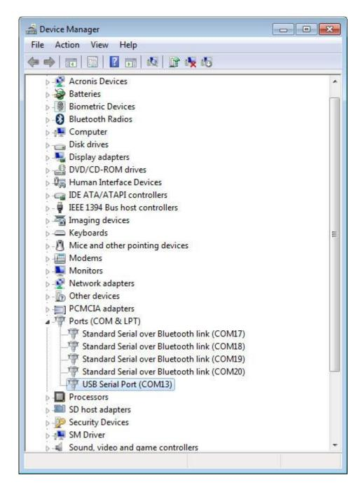
Note: The USB Light will on the ZUSB communications module will only illuminate if the virtual COM port driver is properly installed.
