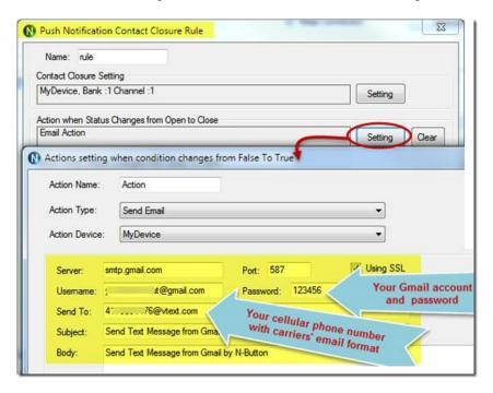
**3.** After finishing all above settings, all recipients will receive an email once the contact closure input on the board changes state. To test, close the contact input on the push notification board and check your email
